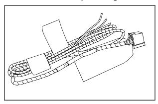
This harness may be included with your vehicle as part of the heavy-duty trailer wiring package.
